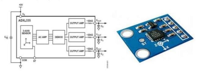
Fig.5. Internal Structure of ADXL335
