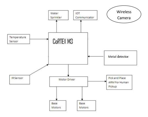
Fig1: Block diagram of the Robot.
