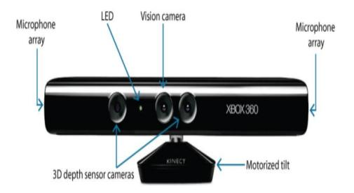
Fig.2. Components of Kinect sensor
