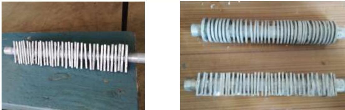
Fig.2 Fabrication of fins
