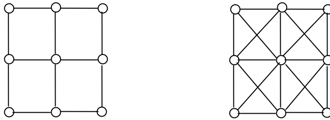
Figure 1: Graph representations of a 3 x 3 matrix with a 4-connected (left) and a 8-connected (right) neighborhood [5].
