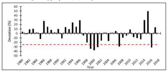
Fig. 4: Percentage deviation of precipitation from normal for Jhelum Basin during 1980-2017 (lower threshold of drought i.e. 25% in red).
