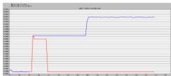
Fig. 7. Delay when traffic is rerouted using TE technique
