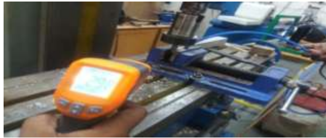
Figure 4: Setup of cutting using the vortex tube to cool
