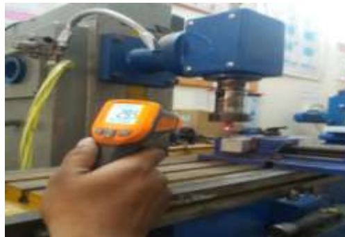
Fig 2: setup of Cutting without coolant
