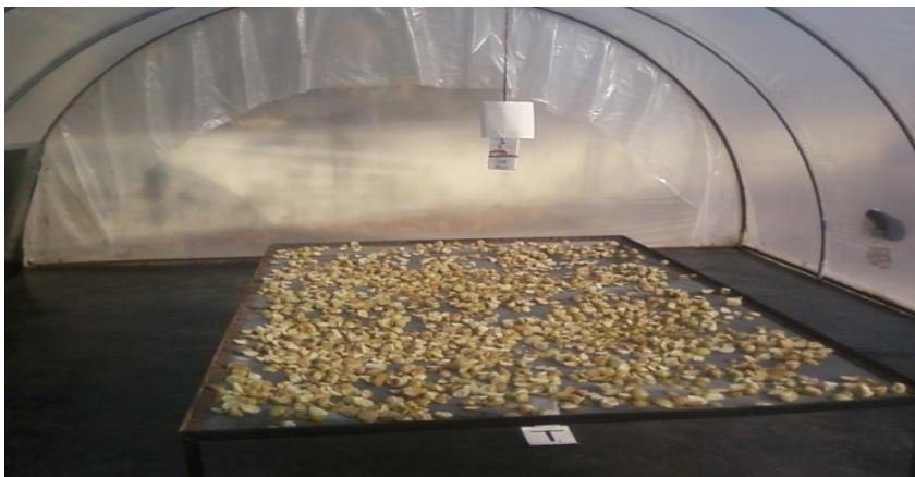
Figure: Measurement of temperature and relative humidity in solar tunnel dryer loaded with Amla (Indian gooseberry)
