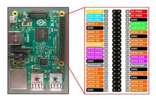
Fig 3.8.2 Raspberry pi 3-pin diagram
