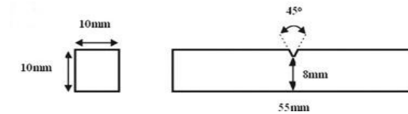
Figure 8. The Specimen dimensions for Impact test
