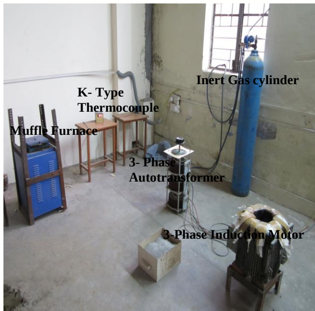
Figure 1. Experimental set up of Electromagnetic stir casting process
