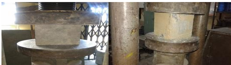
Fig.2 Compressive Strength Test of concrete
