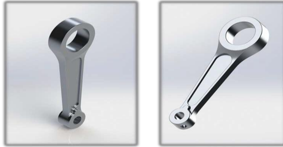
Fig:CAD Model of connecting rod
