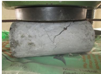
Fig 9: Testing of Split Tensile Strength of Beam Of M-20 Grade Concrete
