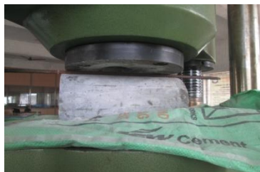
Fig 8: Testing of Split Tensile Strength of Beam Of M-20 Grade Concrete
