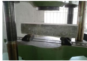
Fig 5: Testing of Flexural Strength of Beam Of M-20 Grade Concrete
