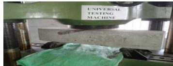
Fig 6 : Testing of Flexural Strength of Beam Of M-20 Grade Concrete
