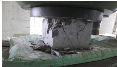
Fig 3: Testing of Cube to find Compressive Strength Test
