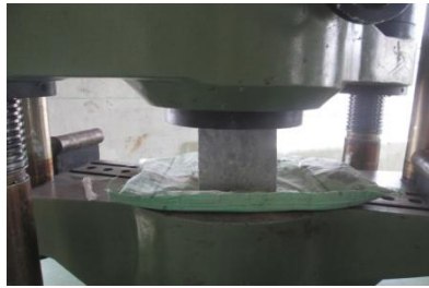
Fig 2: Testing of Cube to find Compressive Strength Test
