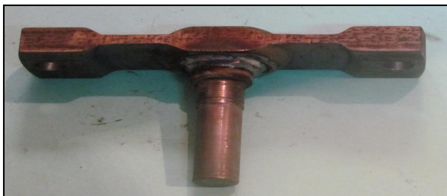
Fig. 11: Design of Yoke 18mm thickness for testing
