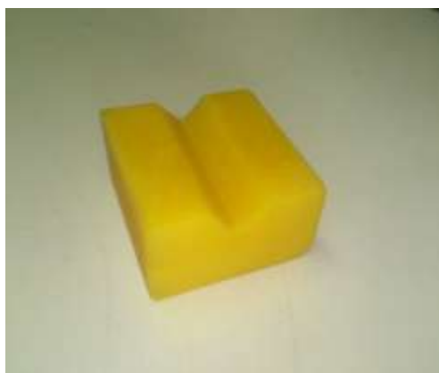
Figure 3.1 Die machined from polyurethane
