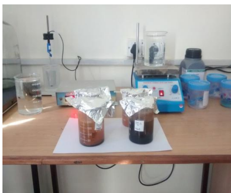
Figure 2: Experimental set up for electroless Ni-P-TiO 2 -ZrO 2 nano-composite coatings
