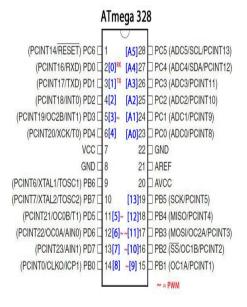
Figure 2: Pin diagram
