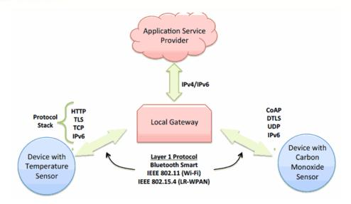
Figure 4. Device-to-gateway communication model diagram.
