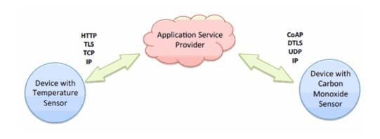
Figure 3. Device-to-cloud communication model diagram.
