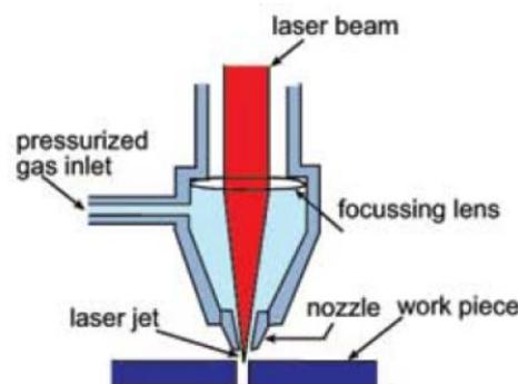
Figure 1: Basic principal of Laser Cutting
