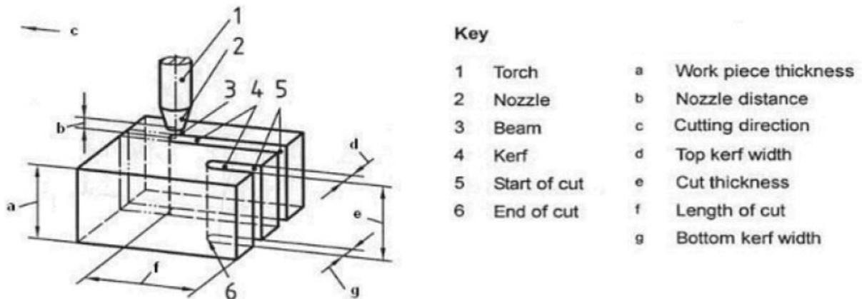
Figure 2: Term related to the cutting process of workpiece
