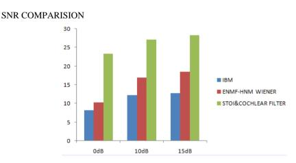
Figure4: Output SNR comparison for IBM, ENMF-HNM, STOI & Cochlear filter
