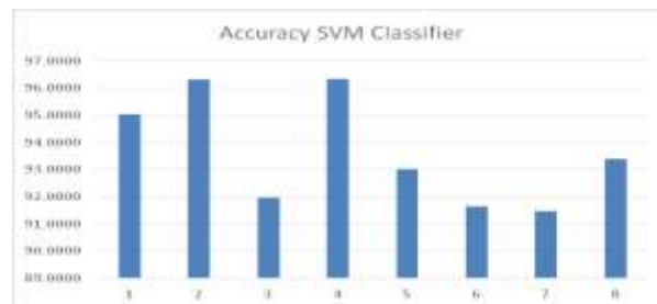
Fig 13: Accuracy rates (%) for SVM Classifier, minimum accuracy of SVM is for the 7 th subset and maximum is for 2 nd subset of data with average accuracy about 93.5%
