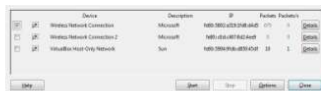
Fig 3: Selecting Packet Interface in Wire shark
