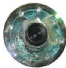
Fig. 2 IR illuminator with camera
