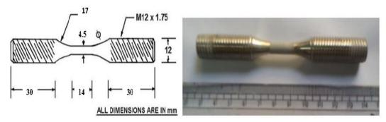
Fig 2: Schematic view of LCF sample
