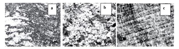
Fig 6: Optical micrographs from cylindrical surface of LCF samples tested at 550°C, (a & b) NaCl coated samples, (c) uncoated sample.
