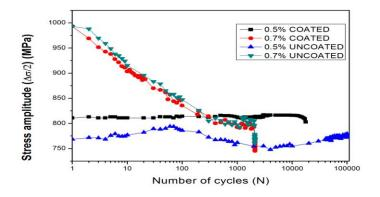
Fig 5: Cyclic stress response curves of alloy IN718 at 550°C for coated and uncoated samples
