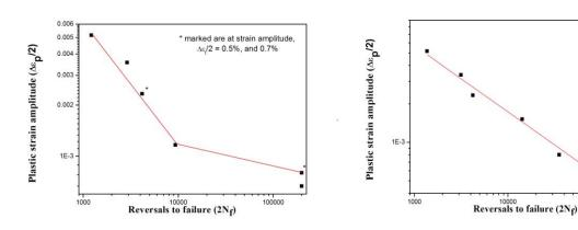
Fig 4: C-M plot (a) for uncoated sample at 550°C (b) for NaCl coated sample at 500°C [4]
