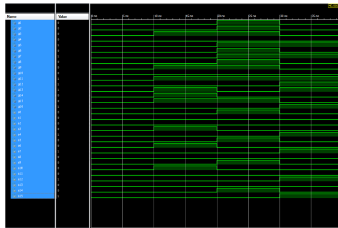
Output waveform of carry skip 1digit BCD adder
