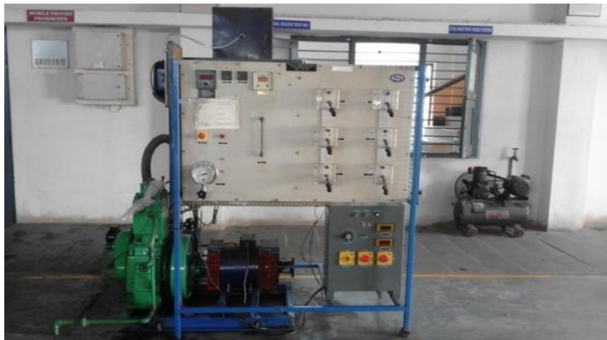
Fig.2: 4 Stroke single cylinder diesel engine set up with generator loading
