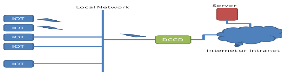
Fig. 4: Block Diagram of Beaglebone Board based Data concentrators for connected Devices
