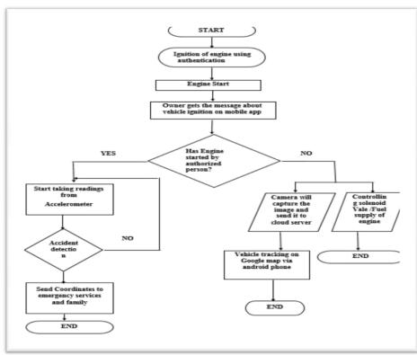
Figure 2 system flow diagram
