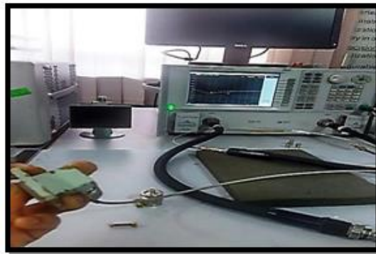
Fig. 8: electrical testing for reflection loss calculation, S_{11}
