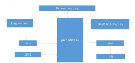
Fig3 Functional block diagram of transmitter system
