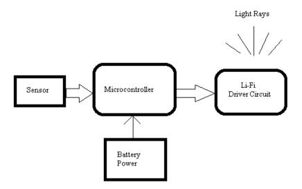
Fig 5 Li-Fi based Wireless Sensor Node
