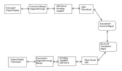
Fig 1 The Basic Block Diagram of the System.
