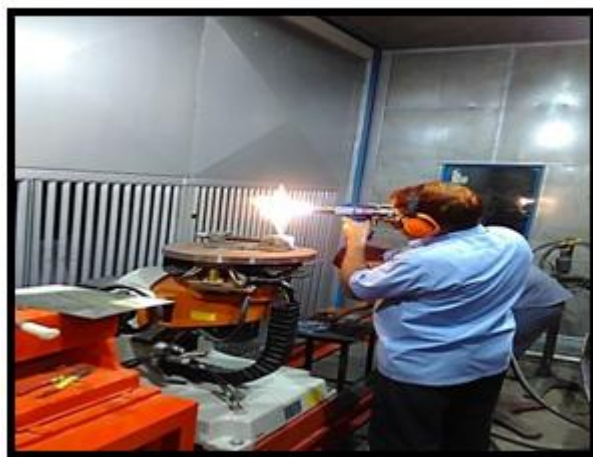
Fig. 2 : experimental flame spray at MEC Jodhpur
