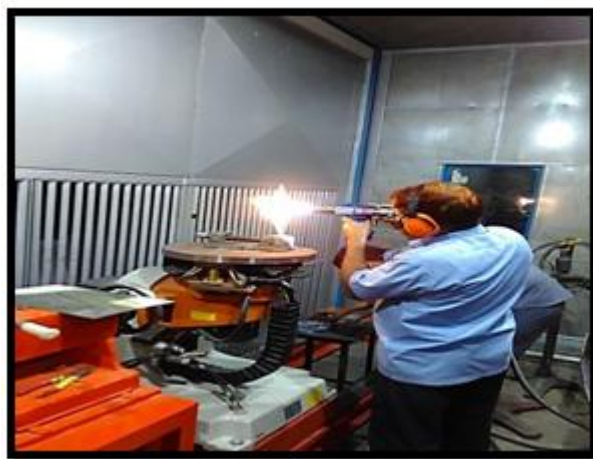
Fig. 2 : experimental flame spray at MEC Jodhpur
