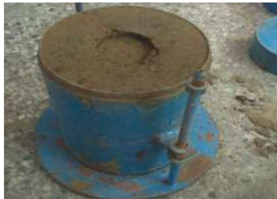
Sample for CBR Test
