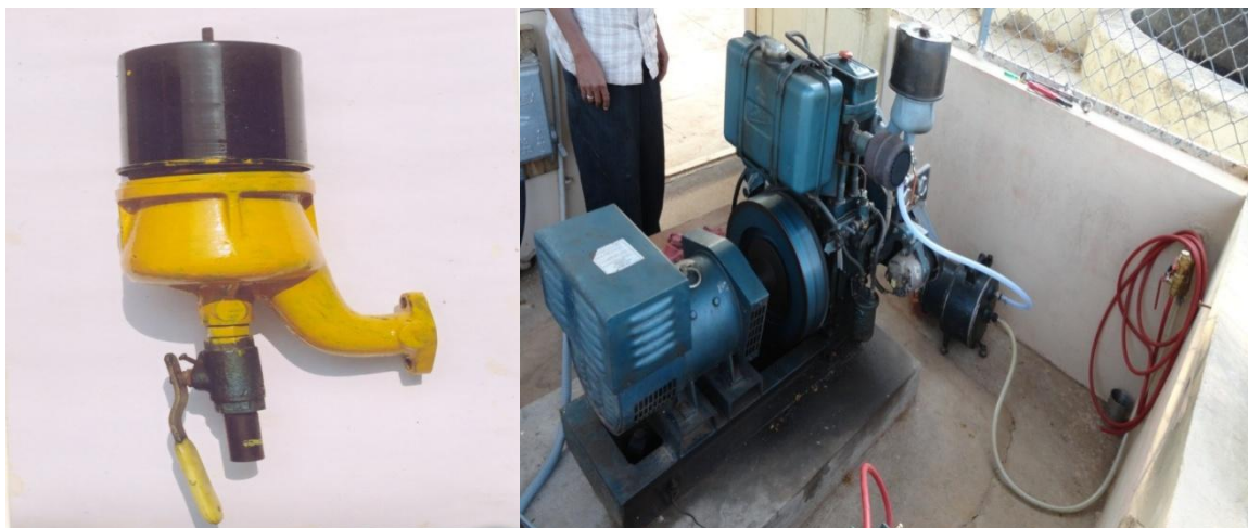
Fig. 1. Mixing chamber and experimental set up for duel fuel engine
