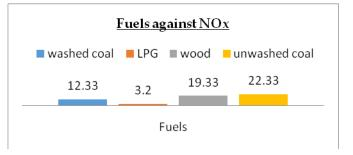
Fig 5 shows fuel against nitrogen oxides
