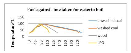
Fig 7 fuel against the time taken for water to boil
