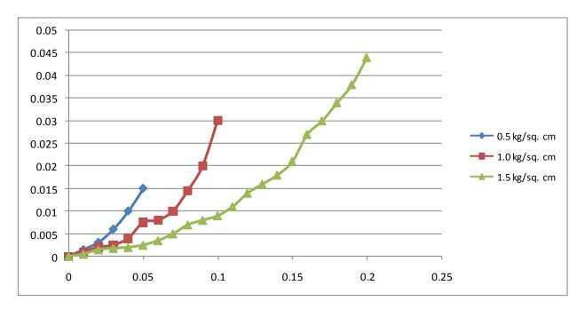
Figure 5: Shear Load v/s Shear Strength for Simple Soil
