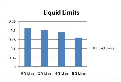
Figure 1: % Lime v/s Liquid Limit
