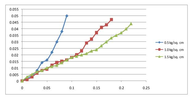
Figure 7: Shear Load v/s Shear Strength for (Soil + 4 % Lime)
