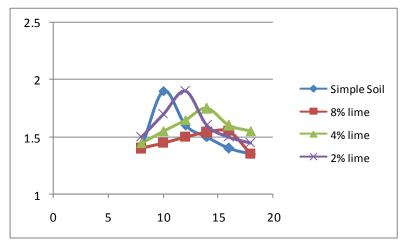
Figure 2: Water content % v/s Dry Density
