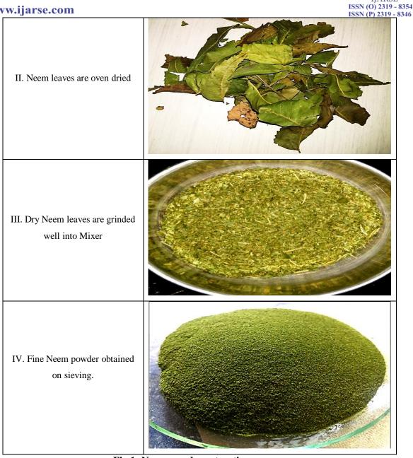
Fig 1: Neem powder extraction process
