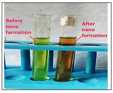
Fig 2: Color testing for AgNPs colloidal solution
