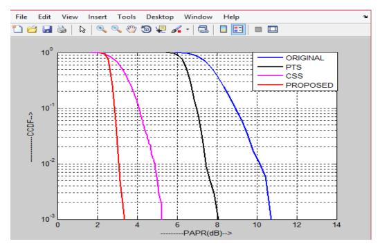
Figure 4. Comparison of PAPR values of Proposed method with previous methods
