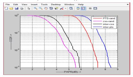
Figure 2. Comparison of the PAPR reduction performance between the conventional PTS scheme and the CSS scheme when N = 128 and U = 64.
