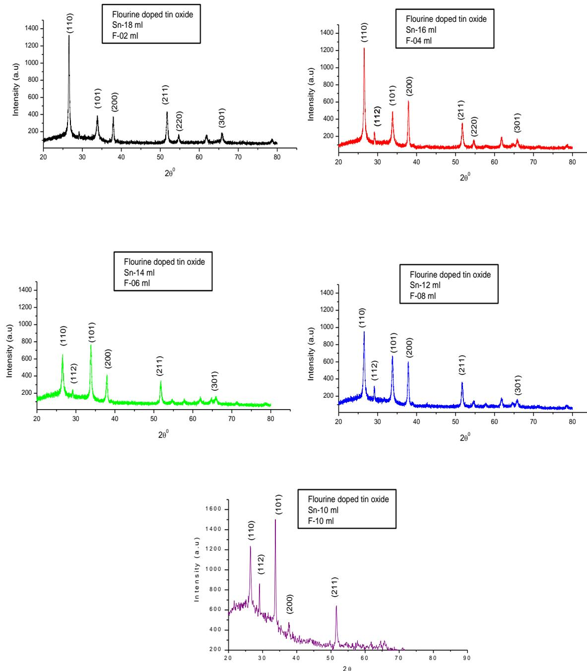
Fig. 2 XRD patterns of fluorine doped tin Oxide (SnO<sub>2</sub>: F) thin films.
