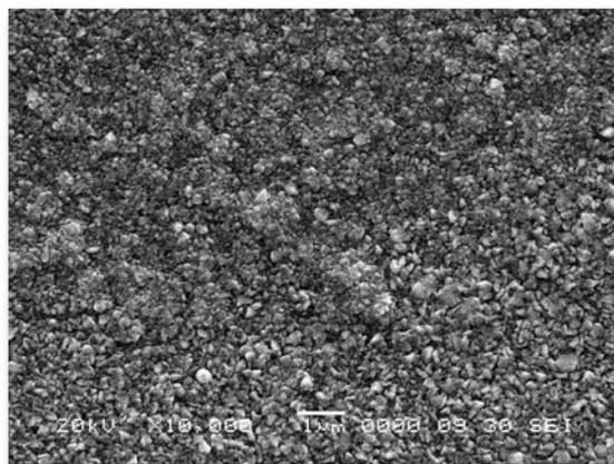
Fig 3. Typical SEM micrograph of SnO<sub>2</sub> thin films.
