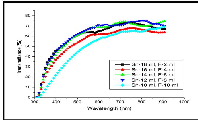
**Fig5: Optical Transmittance against wavelength at different Fluorine concentration of the SnO<sub>2</sub> thin films.**
