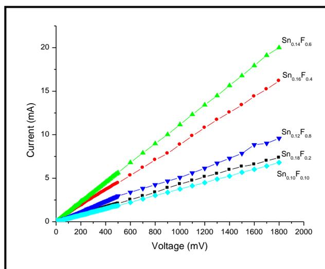
Fig.6 .28 I- V curve of SnO<sub>2</sub>: F thin films as a function of wavelength for different fluorine doping.
