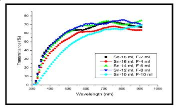
Fig5: Optical Transmittance against wavelength at different Fluorine concentration of the  $SnO_2$  thin films.
