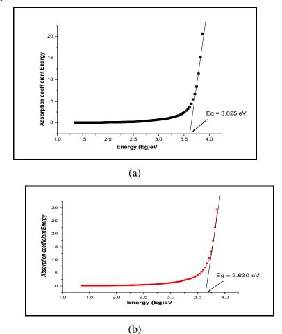
Fig.6 (a & b) typical plot of absorbance coefficient Vs. Photon energy for SnO2: F & SnO2 thin films.
