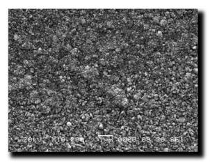
Fig 3. Typical SEM micrograph of SnO<sub>2</sub> thin films.
