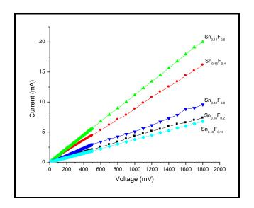
Fig. 6.28 I-V curve of SnO2: Fthin films as a function of wavelength for different fluorine doping.
