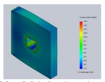
Fig.3 stress distribution of rectangle cross section area
