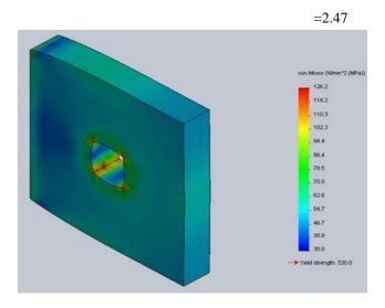
Fig.2 stress distribution of square cross section area
