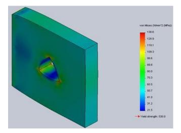
Fig.4 Stress distribution of triangle cross section area TABLE 5 Values of Triangle Hole After Simulation
