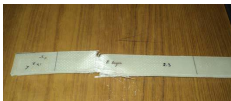
Figure .4 : Specimen failure after tensile test
