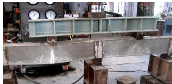
Figure 6: Failure of the beam by tensile rupture
