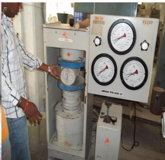
Fig.6 placing a specimen in split tensile testing machine
