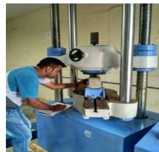
Figure 3.5: Performing Flexural Strength Test
