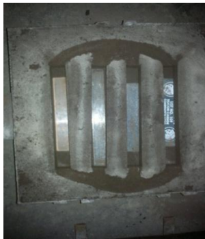
Fig1. Mold preparation with Chill being melted
