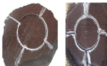
Sintered Ceramic Parts and Separation from the redundant material (Fig-5)
