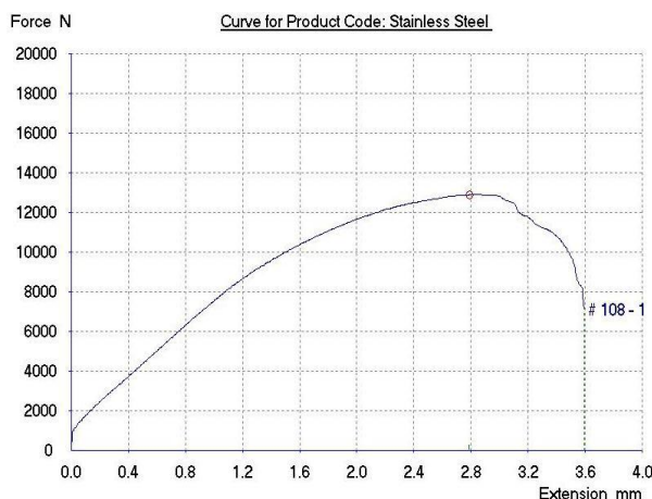
Graph 4.3: Force vs. Extension curve for Sample 1
