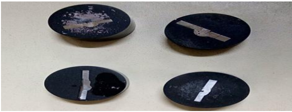
Fig.3.3: Prepared mould to use for microstructure study
