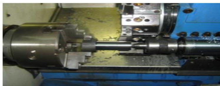
Fig.2 Turning Process in CNC Lathe Machine
