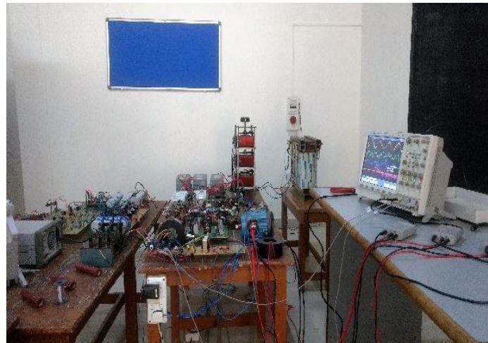
Fig.5a Experimental set up photograph of 3-level inverter circuit
