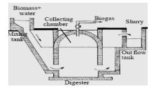
fig8: fixed dome biogas plant
